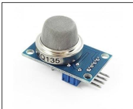
**Gambar 2.6 Sensor Gas MQ-135**
