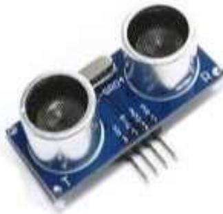
**Gambar 2. 12** Sensor UltraSonic/HCSR-04
