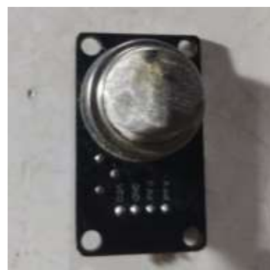
Figure 7. Condition of MQ-8 Hydrogen Sensor after Overheating
