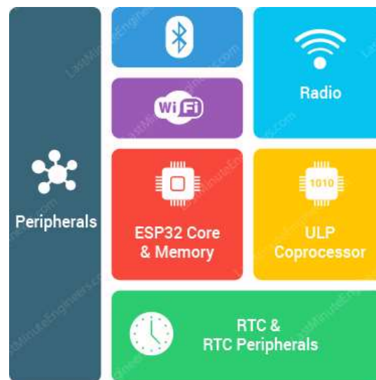
Gambar 2. 2 Diagram Blok Chip ESP32
