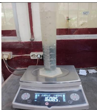
Berat Pycnometer + agregat + air
