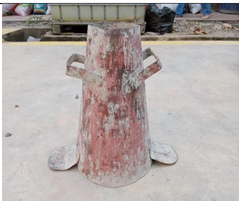
Corong Slump Test
