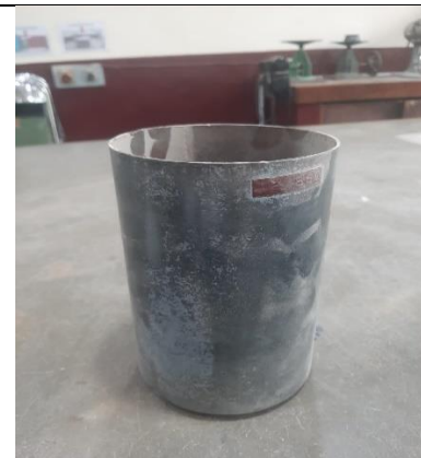
Bejana Silinder Bobot isi Agregat
