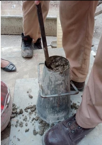
Slump Beton didalam Bejana Kerucut
