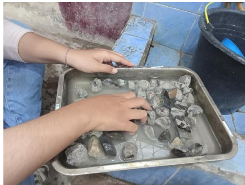
Gambar 4.2 Pencucian Benda Uji
