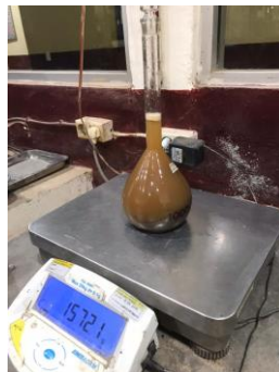
Gambar 5.4 Penimbangan Pycnometer + Agregat Halus + Air
