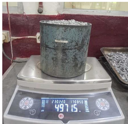
Gambar 8.6 Penimbangan Agregat Kasar
