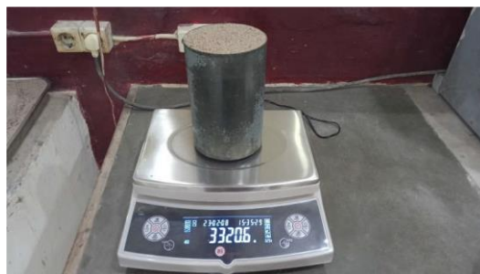
Gambar 9.3 Penimbangan Bejana Silinder + Agregat Halus
