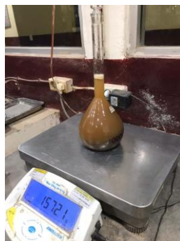
Gambar 5.4 Penimbangan Pycnometer + Agregat Halus + Air
