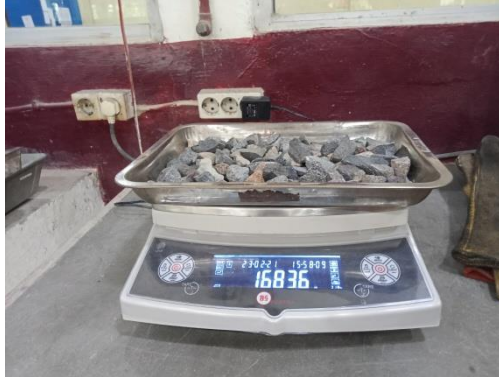
Gambar 6.1 Penimbangan Agregat kasar
