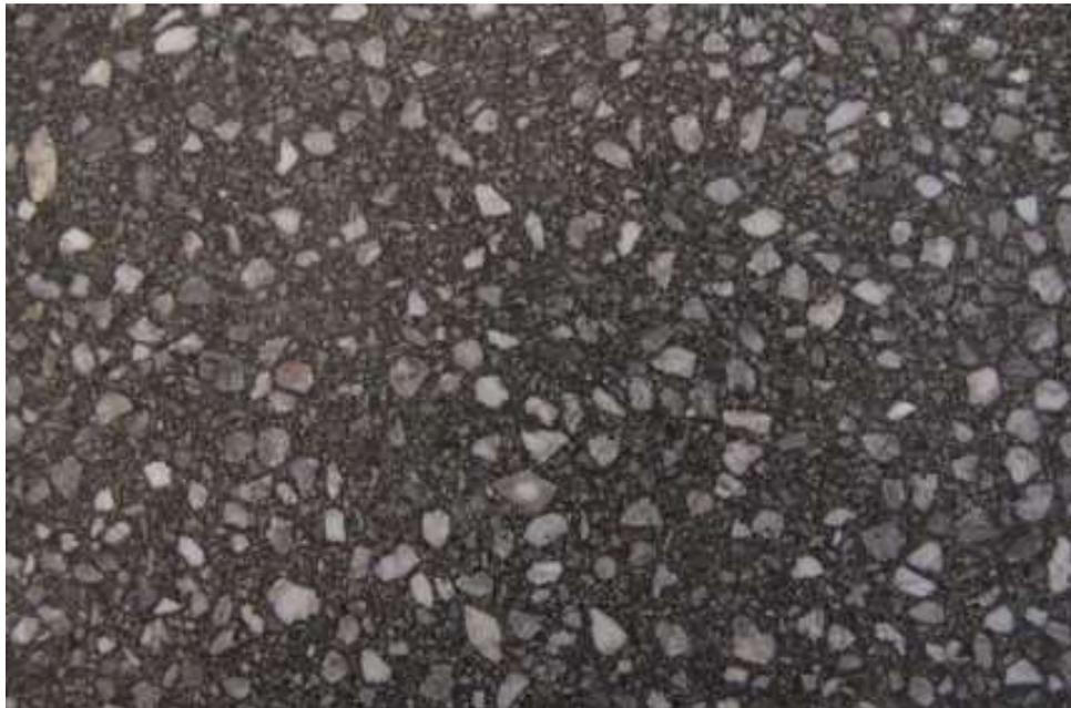
**Gambar 2.17** Pengausan agregat (*polished aggregate*)
