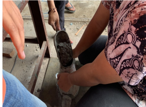
Proses pengujian slump test
