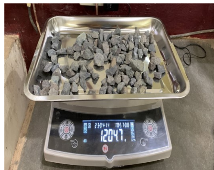
Proses penimbangan kadar lumpur agregat kasar kering oven
