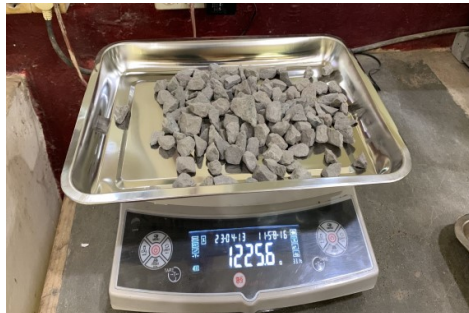
Proses penimbangan kadar air agregat kasar kering oven
