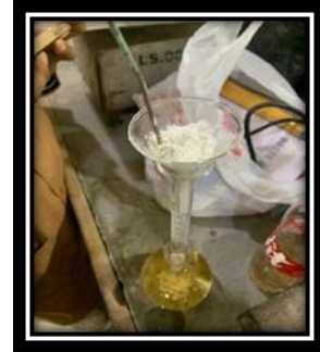
Penimbangan Pycnometer + Air + Serbuk Gypsum
