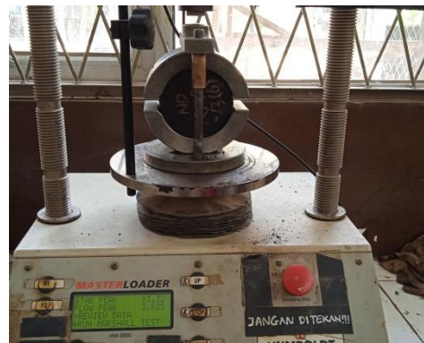
Gambar 19.6 Proses Uji Marshall
