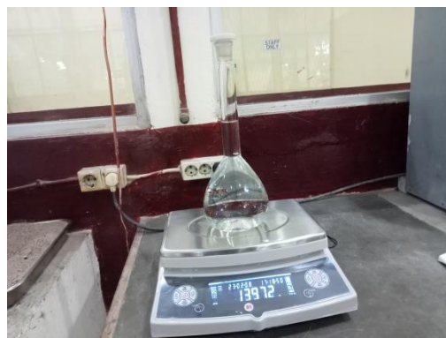
Gambar 9.3 Proses Penimbangan Pycnometer Kosong dan Pycnometer + Air
