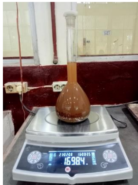
Gambar 9.6 Penimbangan Pycnometer + Agregat Halus (Pasir) + Air
