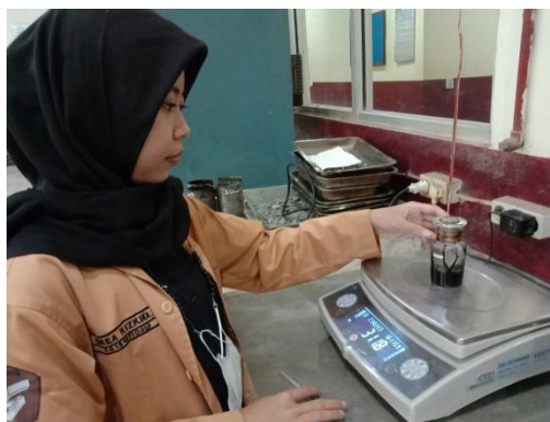
Gambar 14.7 Penimbangan Piknometer + Aspal + Air
