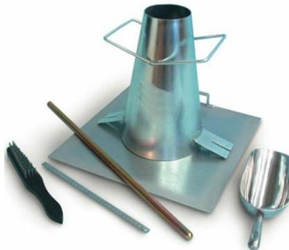
Gambar 2. 5 Alat Slump Beton
