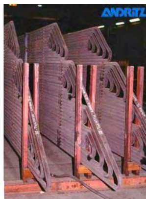
Gambar 2. 6 Gambar pipa Superheater (Adrian et al., 2016)
