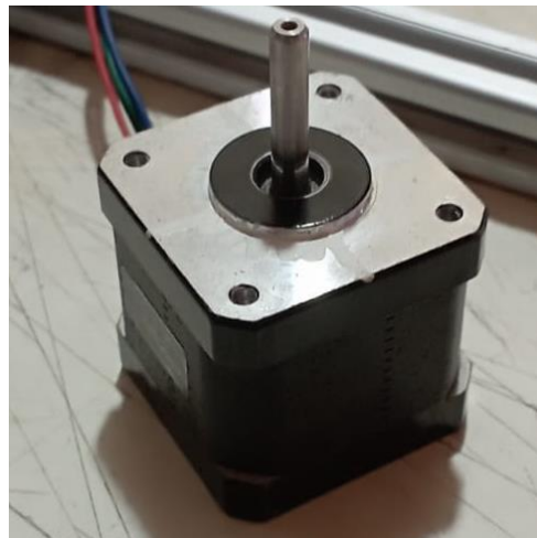
Gambar 2.2 Motor Stepper (Rafli,2023)
