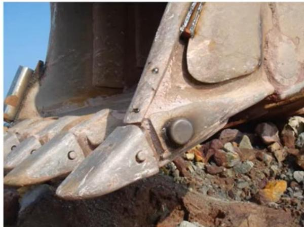
Gambar 2.9 *Wear Bucket Excavator*
