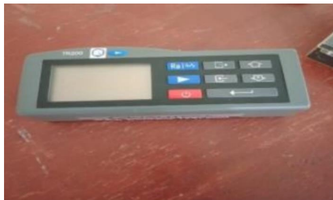
Gambar 2.5 Alat Ukur Kekasaran ( Roughness Tester ) TR200
