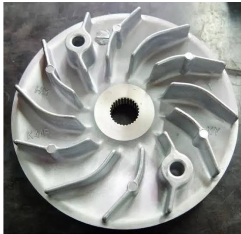
Gambar 2. 16 Primary fixed sheave (Marsudi, 2017)
