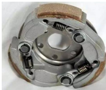
Gambar 2. 32 Clutch carrier (Marsudi, 2017)
