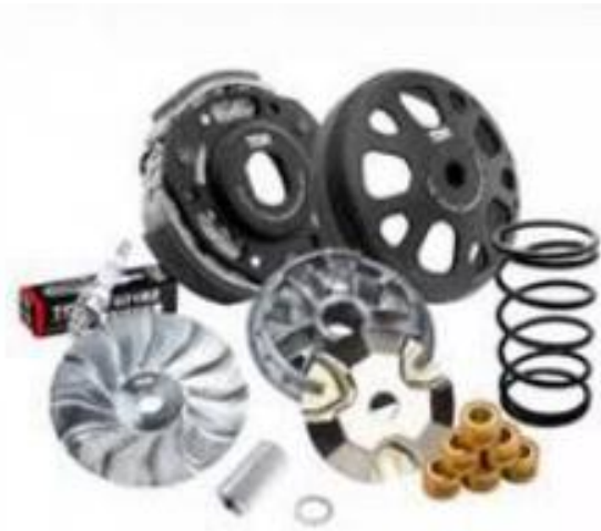
Gambar 2. 17 Primary sliding sheave (Marsudi, 2017)
