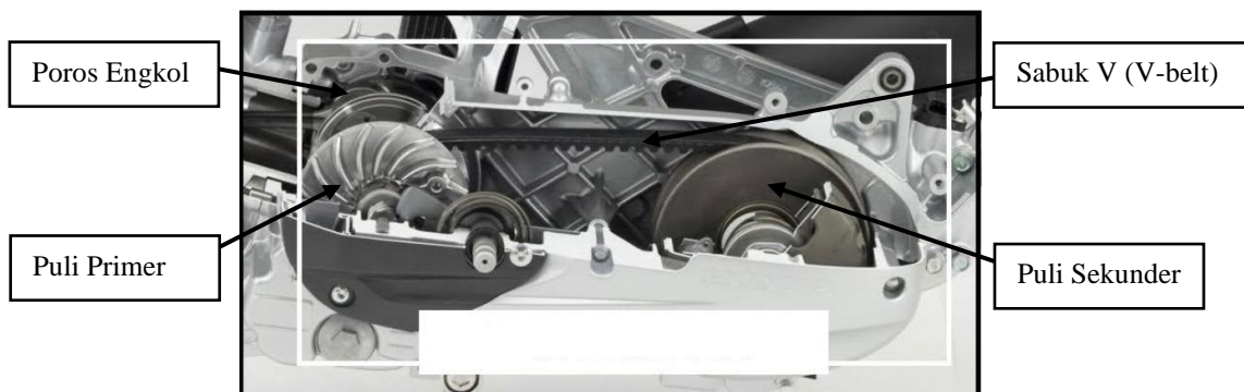
Gambar 2. 1 Continuously Variable Transmission (Marsudi, 2017)
