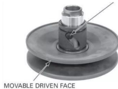
Gambar 2. 30 Secondary fixed sheave (Marsudi, 2017)
