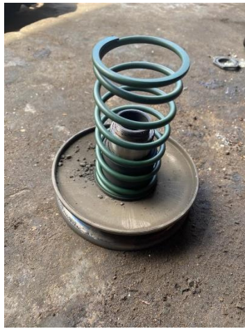
Gambar 6. Spring BRT Kekerasan Tekan 10-15%
