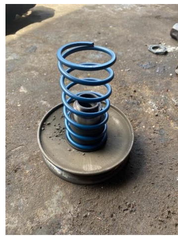
Gambar 7. Spring BRT Kekerasan Tekan 20%
