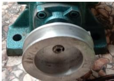
Gambar 2.8 Pulley Gear Box
