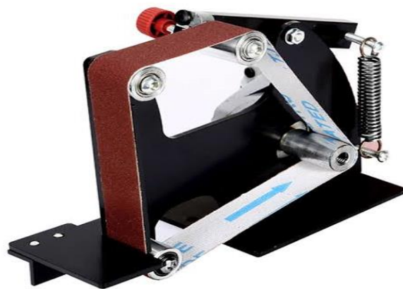
Gambar 2.2 Mesin Amplas Sabuk (Trade, 2023)
