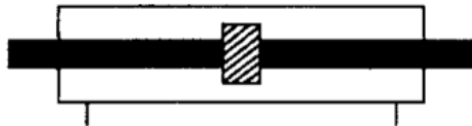
Gambar 2. 8 Through rod pneumatic cylinder (RK Rajput, 2007)
