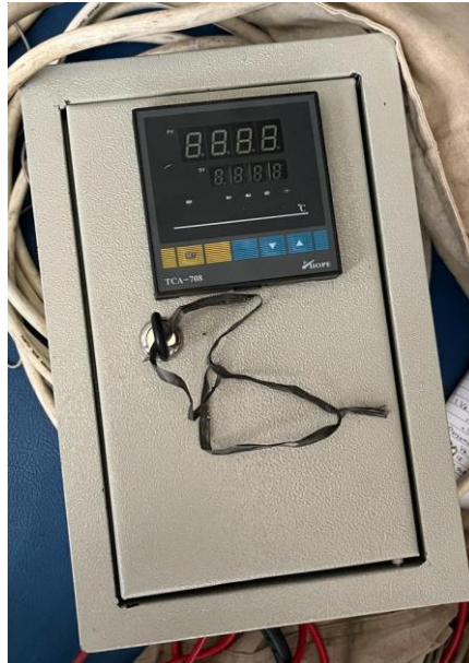
Gambar 2.5 Termometer Control ( Fatur, 2023)
