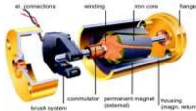
Gambar 2. 2 Motor listrik DC (Otoflic.com, 2015)
