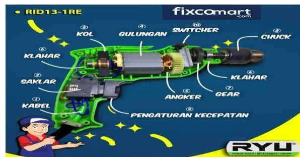
Gambar 2. 17 Bagian-bagian Bor Tangan ( https://fixcomart.com/blog-detail 2018)
