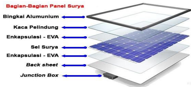
Gambar 2.10 Bagian-bagian Panel surya
