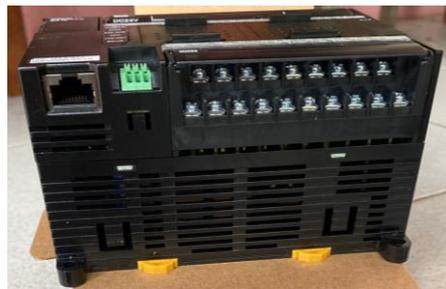
**Gambar 2.2** *Programmable Logic Control* omron tipe CP1L-E
