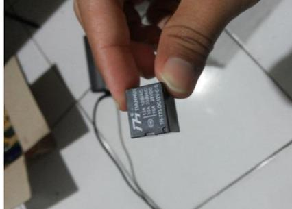
**Gambar 2.5 Relay SPDT**
