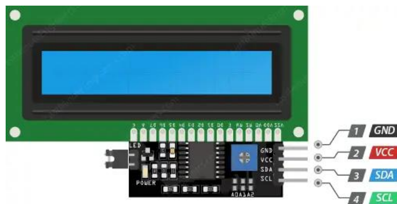
Gambar 2. 12 Pinout LCD I2C
