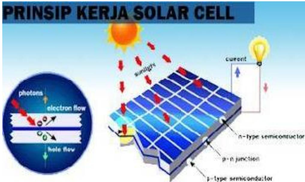
**Gambar 2. 4** Prinsip Kerja Solar Cell
