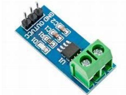
Gambar 2.9 Sensor Current
