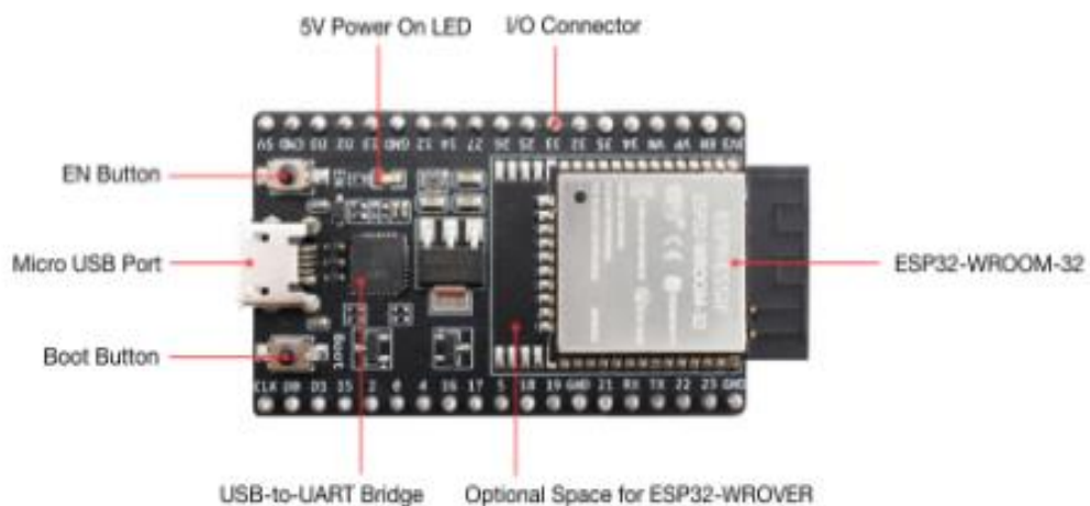
ESP32-DevKitC V4 with ESP32-WROOM-32 module soldered
