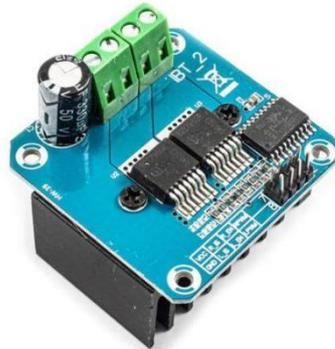
**Gambar 2.9** Drive Motor bts7960
