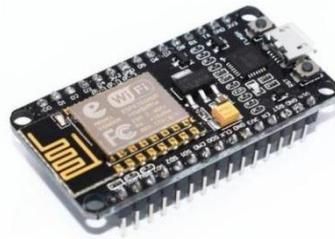
**Gambar 2.5** ESP NodeMCU
