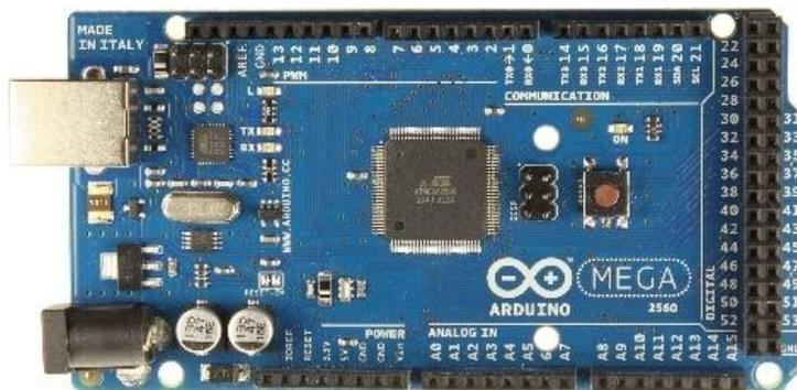
**Gambar 2. 10** Arduino Mega 2560
