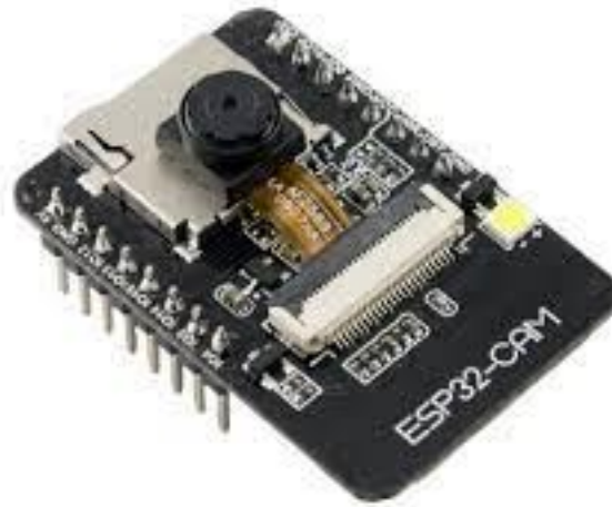
Gambar 2.2 ESP32-CAM Sumber : pschatzmann.ch
