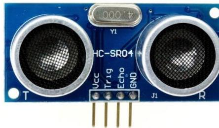
**Gambar 2. 1** Sensor Ultrasonik [4]
