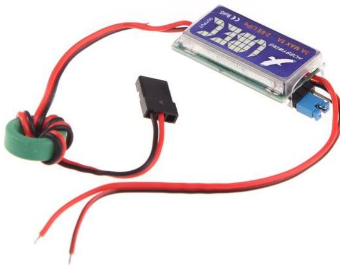
Gambar 2. 21 UBEC ( Universal Battery Elimination Circuit )
