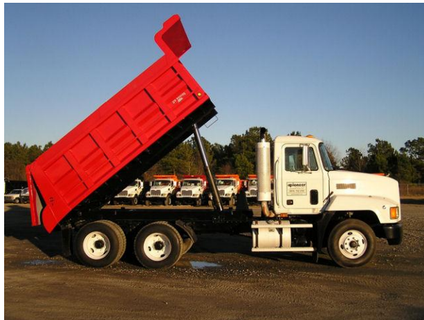
Gambar 2.1 Dump Truck Rear Dump
