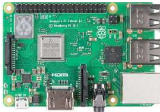
Gambar 2. 4 Tampak Depan Raspberry Pi 3 Model B+ [8]. kabel Ethernet [8].
