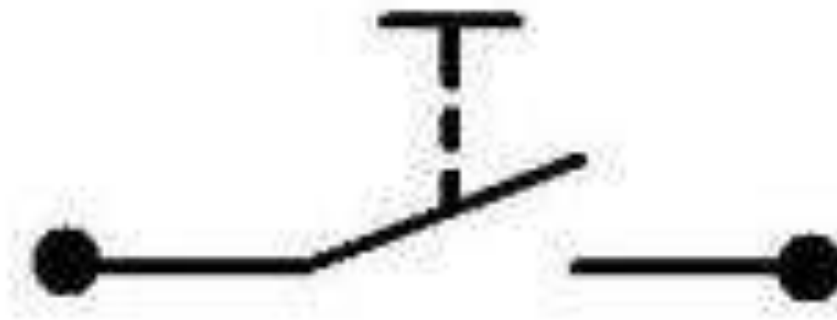
Gambar 2.18 Simbol Limit Switch
