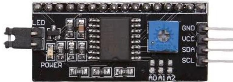
**Gambar 2.13** Inter Integrated Circuit (I2C)
