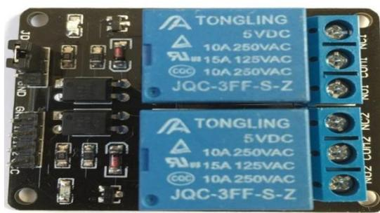
**Gambar 2.21 Module Relay 2 Channel**
