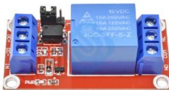
**Gambar 2.20 Module Relay 1 Channel**
