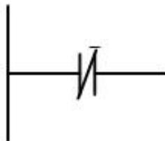
**Gambar 2.6 Ladder Diagram simbol Load Not ( LD NOT )**
