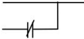
**Gambar 2.10 Ladder Diagram simbol OrNot ( OR NOT )**
