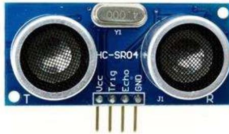
**Gambar 2.7** Sensor Ultrasonik HC-SR04
