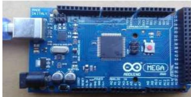
**Gambar 2.8** Arduino Mega 2560
