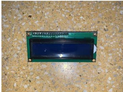
**Gambar 2.1** LCD i2c 16 x 2<sup>[4]</sup>
