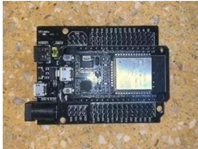
**Gambar 2.12** NodeMCU ESP32 [49]
