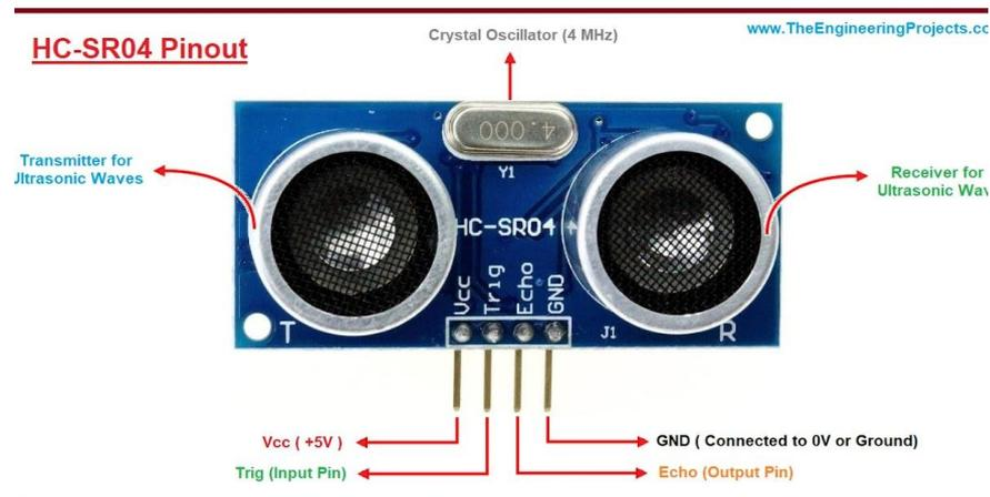
**Gambar 2.4** Sensor ultrasonic HC-SR04Sumber : <https://tinyurl.com/mrwzm7ms>
