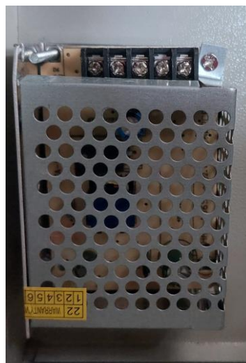
Gambar 2. 7 Power Supply Switching [12]
