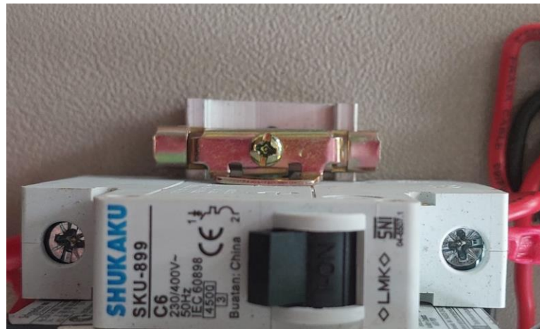
Gambar 2. 10 MCB (Miniatur Circuit Breaker) [15]
