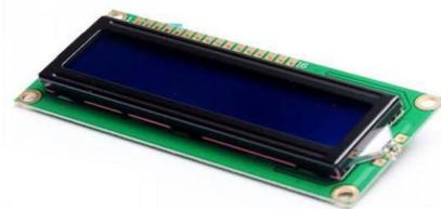
**Gambar 2. 12** *Liquid Crystal Display*
