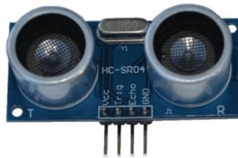
**Gambar 2. 5** Sensor Ultrasonik HC-SR04
