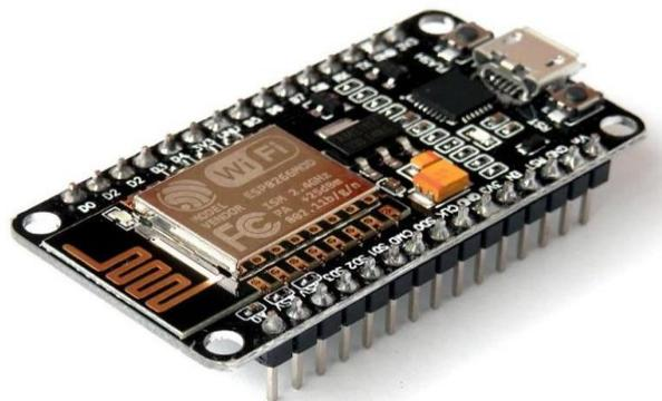
**Gambar 2.3** NodeMCU ESP8266
