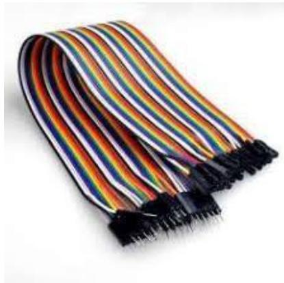
**Gambar 2.16** Kabel Jumper [18]
