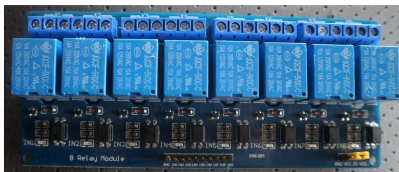
**Gambar 2.8** Relay Module 8
