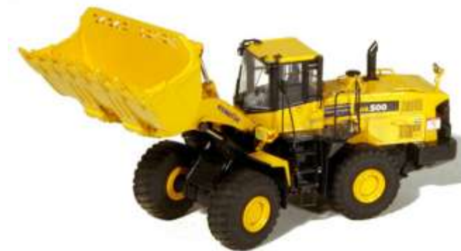
Gambar 2.12 Bucket in tilt Position
