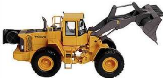
Gambar 2.13 Bucket in Dump Position
