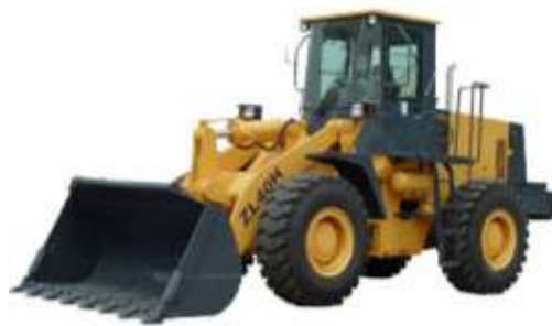
Gambar 2.14 Bucket in Hold Position
